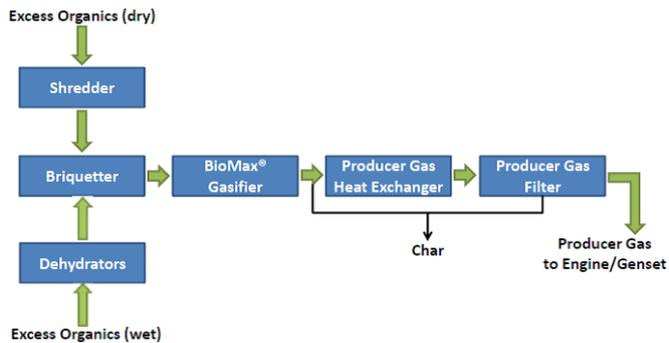
**Figure 1. Block diagram of the flow path for materials and gas through HEDWEC.**
