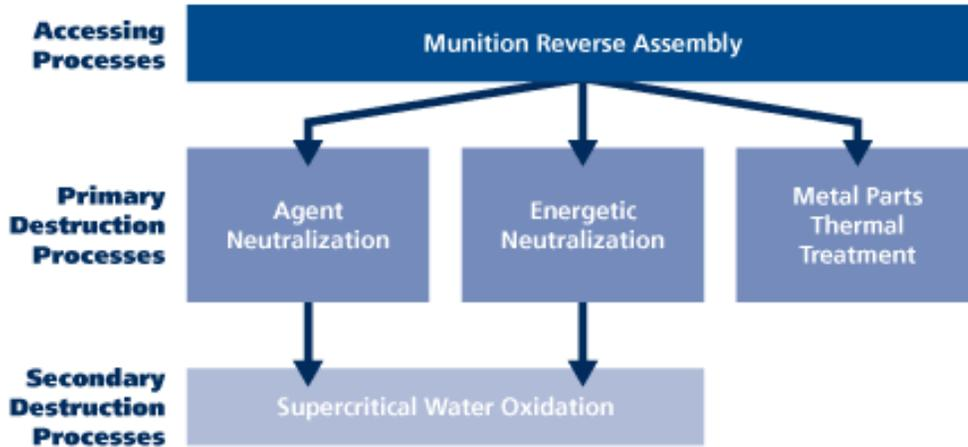
Figure 2: Layout of Chemical Agent Neutralization followed by Supercritical Water Oxidation used at the Blue Grass Army Depot.<sup>5</sup>
