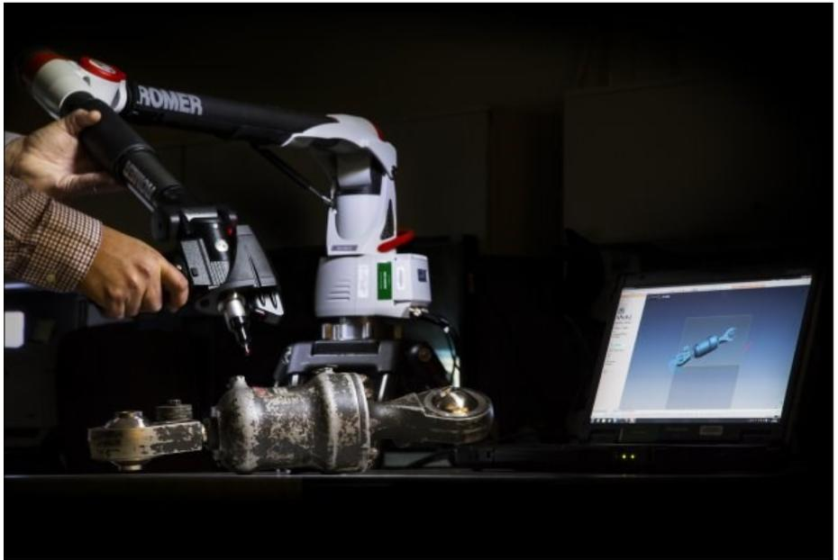
3-D scanning technology is used by the Army to create models for visualization, prototypes and reverse engineer existing technologies. (Photo courtesy of the U.S. Army)
