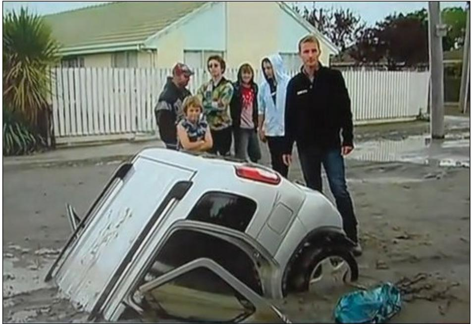
**Figure 2: Liquefaction following the Christchurch Earthquake in New Zealand in 2011. While usually not directly hazardous to humans, liquefaction complicates transportation and can damage buildings and infrastructure. (Image courtesy of the Pacific Northwest Seismic Network/Released)**
