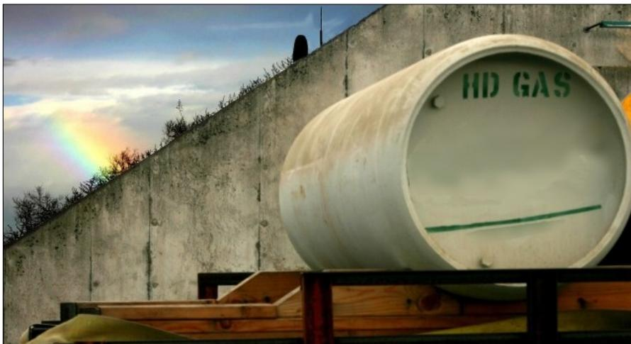
A bulk container of mustard agent is loaded on a truck outside a storage igloo as it is prepared for transport to the disposal facility. While marked as "gas," chemical agents are actually liquid in storage. Detonation would render the liquid into gas. " (Photo courtesy of the U.S. Army)
