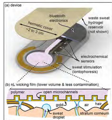
**Figure 1. Diagram of an advanced sweat biosensing device, including integrated localized stimulation of sweat (sweat on-demand), advanced wicking materials to work with tiny nanoliter volumes of sweat, and electrochemical sensors to continuously read biomarker concentrations.**
