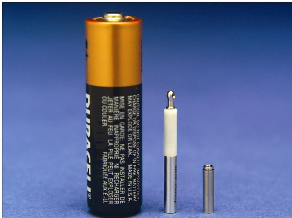
This photo shows a miniature battery next to a bion and a commercial AA battery. The miniature battery used in the bion is 100 times smaller than a AA battery. Researchers are developing new methods for manufacturing miniature batteries. (Photo courtesy of the Department of Energy)
